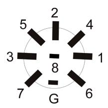
Pin-out for the 8-Pin female DIN connector on the stainless steel wall plate, as viewed from the rear of the connector.
