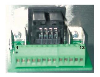
Pin-out for the 13-Pin female DIN on the stainless steel wall plate, as viewed from the rear of the wall plate.
