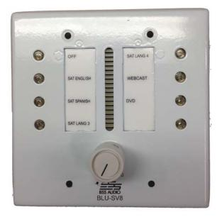
The BLU-SV8T is a source selector/volume control for *BSS Audio London Series Digital Signal Processors.* It is built on a dual gang panel for mounting in a dual gang electrical box. The front side of the control has 8 lighted momentary pushbutton switches for selecting audio, and a pot for adjusting the volume of
